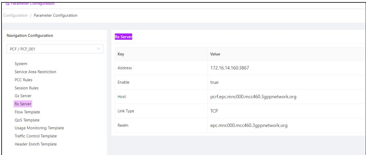
The screenshot shows the 'Parameter Configuration' interface for 'Rx Server' settings. The left sidebar shows navigation for 'PCF / PCF\_001' with 'Rx Server' selected. The main area displays a table with the following data:
