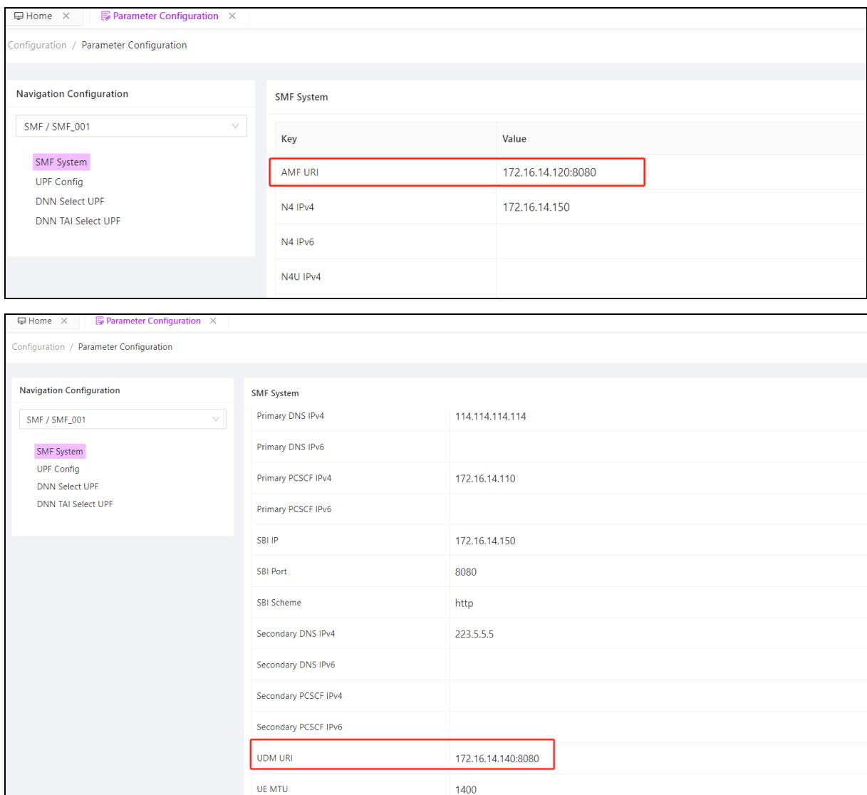
The screenshots show the 'Parameter Configuration' interface for the SMF System. The top screenshot displays the 'AMF URI' configuration, which is set to 172.16.14.120:8080. The bottom screenshot displays the 'UDM URI' configuration, which is set to 172.16.14.140:8080.
