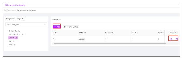
4. **TAI List**: In the TAI List, you can modify, add, and delete TAC corresponding to PLMN, PLMN and TAC correspond to base stations. If the AMF is incorrectly filled, the connection between the AMF and the base station may be interrupted.
